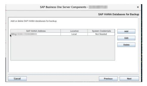
At least one SAP HANA database server must be specified for backup. The SAP HANA database server can be on the same machine (local) as the backup service or on a different machine (remote).
